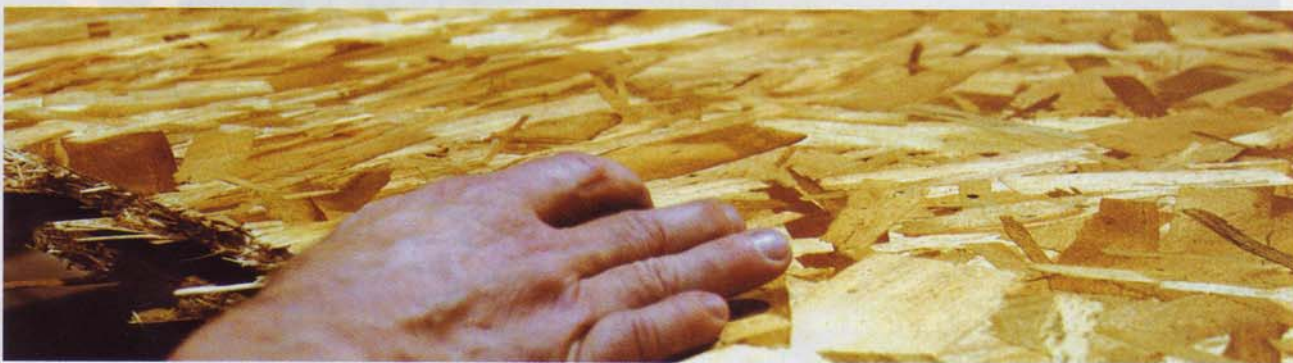
For OSB, the strands for the faces are usually oriented parallel with the longitudinal direction of the panel (machine direction) and the core layers are either cross-oriented or laid random.
